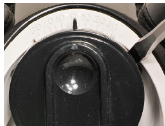
9.2: Use a flat screw driver to pry the flap assembly out as shown
