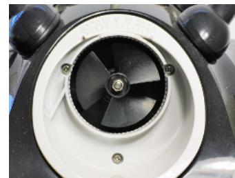
9.3: Snap the flap assembly back after cleaning
