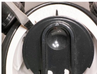
9.1: Remove the flap assembly to clean the dirt or hair on impeller
