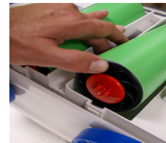
8.3: After cleaning the roller, snap it back in.
